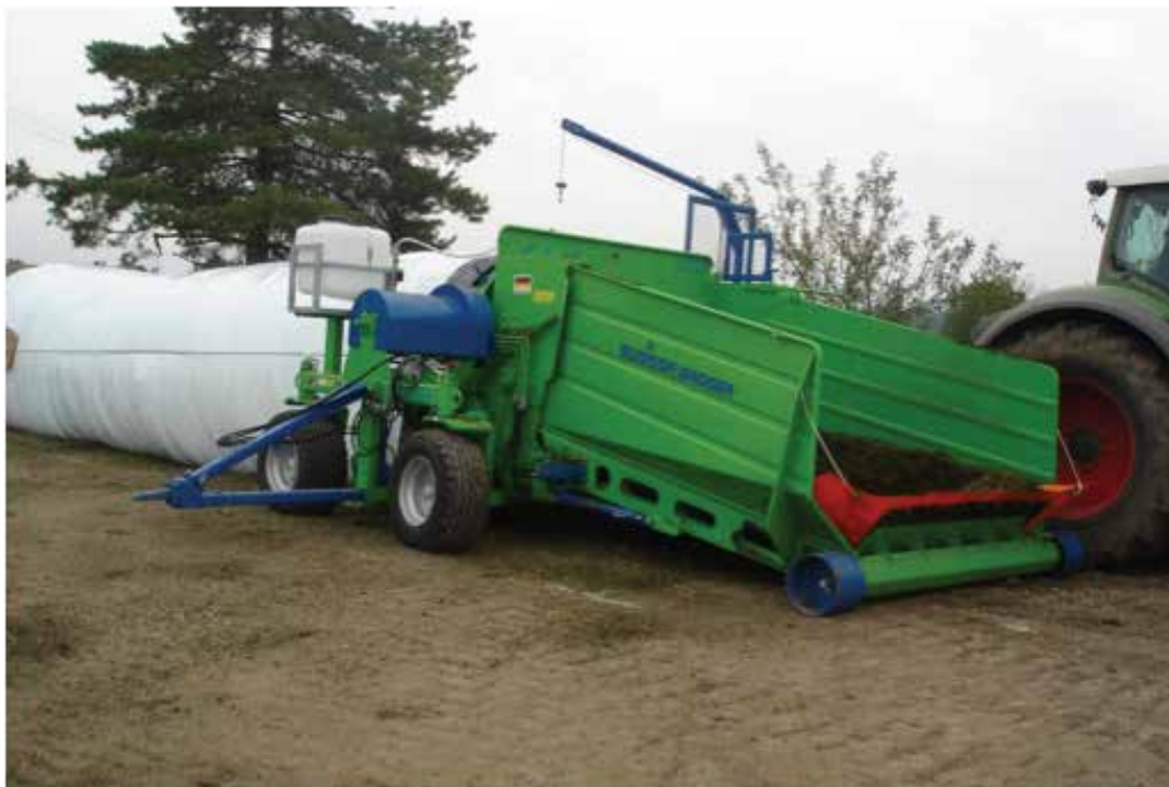
Image 6. Press for compress of biomass into the polyethylene tube for ensilaging.
